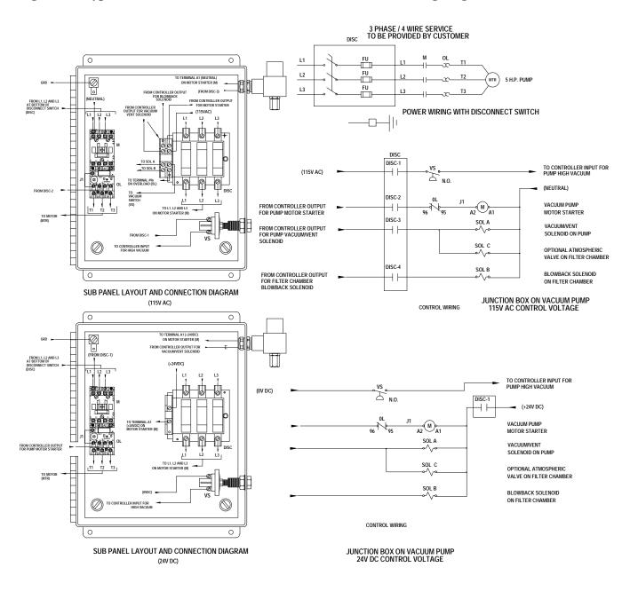
Figure 37: Typical SPD Series Junction Box with Fused Disconnect Wiring Diagram
